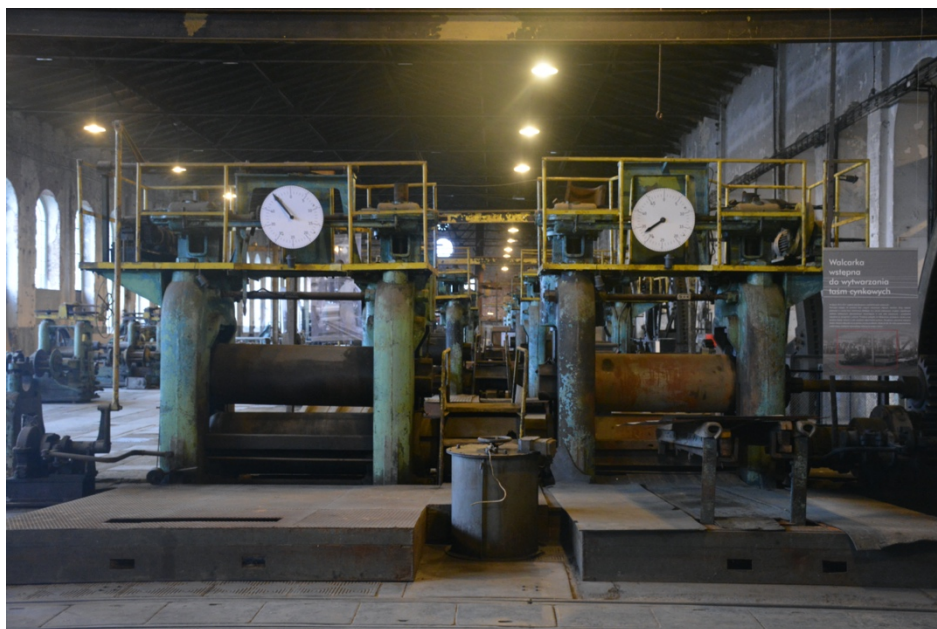
Fig. 1: The interior of the Zinc Rolling Mill hall from 1904. in Katowice with visible zinc sheet rolling mills, 2018. Source: P. Chodak
